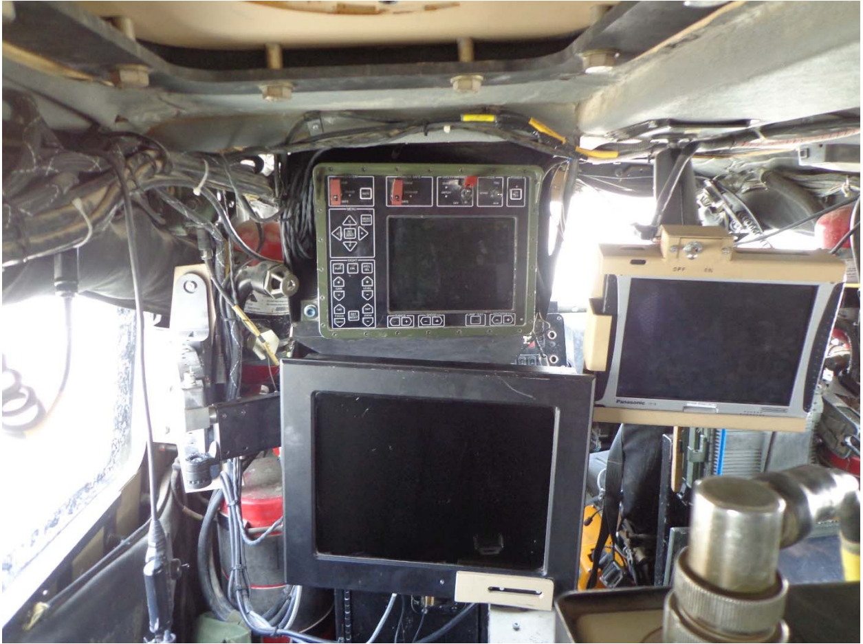
Figure 9: Current crew station includes separate displays for each of the enablers in use, limiting room for future capability growth and creating integration challenges.
